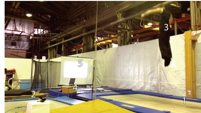
Figure 1. User study setup. 1: trampoline, 2: Kinect depth camera, 3: user, 4: computer, 5: screen
