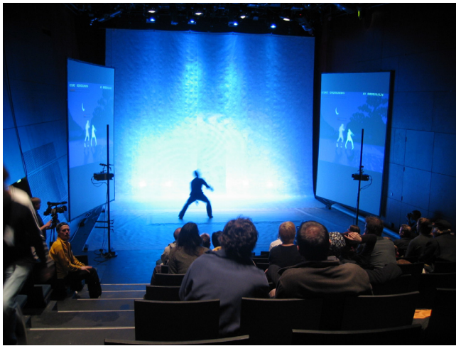
Figure 2. Kick Ass Kung-Fu on stage in a theater. The player moves on a cushioned mat, facing either one of the projected screens. The player sees himself or herself on the screen in a profile view familiar from traditional martial arts games.
