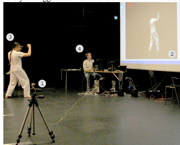
Figure 1. A video mirror test setup, showing camera (1), camera view projected on a screen (2), user (3) and test instructor (4).
